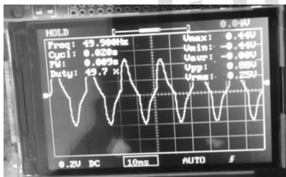
Fig 6 Oscilloscope results for pure PVDF
