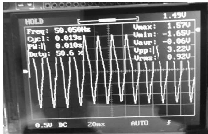
Fig 8 Oscilloscope results for 0.2% CNF with PVDF/TiO 2
